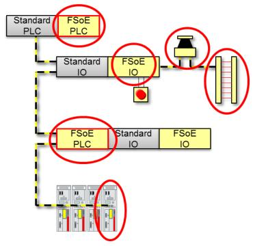
Figure 3: Devices with FSoE interface
