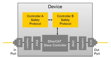
Figure 4: Hardware architecture
