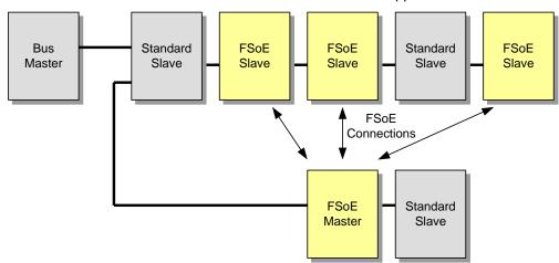
Figure 1: FSoE system architecture
