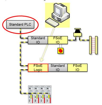
Figure 2: Decentralized Safety Logic approach with Standard PLC
