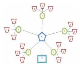
Fig. 3. Architecture of the hybrid WSN-RFID network (T - tags, R - readers, C -coordinator, S - server)
