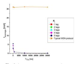
Fig. 6. Average current consumption vs. transmission period
