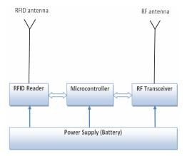
Fig. 2. Architecture of a hybrid RFID reader
