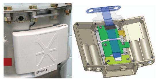
3 Left: prototype tag mounted on Model 9975 drum and right: interior view of tag with metal back plate removed
