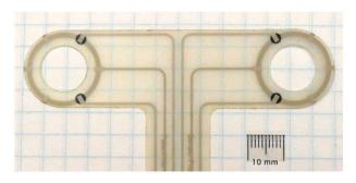
2 Seal sensor for prototype tags
