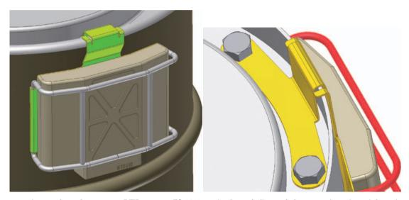
4 Conceptual mounting of prototype RFID tag on ES-3100 packaging: similar variations can be adopted for other drum types
