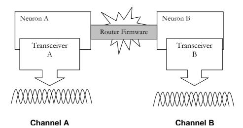
Routers are used to optimize packet traffic on channels. Packets generated on one channel are selectively forwarded to another channel if they contain address information referencing that channel.
