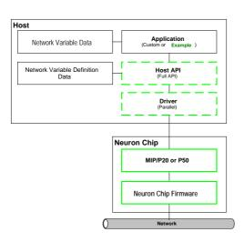
The MIP is delivered as a Neuron C library that allows the NodeBuilder software to include system calls for the MIP. The NodeBuilder is needed to create a ROM image that executes on the Neuron chip.
