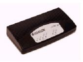
The PCLTA-21 interface for use with PCI-bus PCs is available with FTT10A or TP/XF1250 (1.25Mbps) transceivers.
