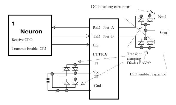
The network connection (NET1 and NET2) is polarity insensitive and therefore either of the two twisted pair wires can be connected to either of these two network connections.
