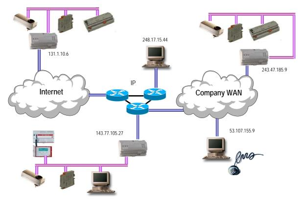
LonWorks Packets are encapsulated within the TCP/IP packets. Every iLon-600 has its own IP address. An Introduction to control networks based on LONWORKS® Technology
