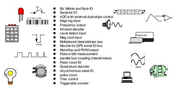
The programming model of the Neuron C language allows the programmer to declare one or more pins as I/O objects. These declarations can be thought of as written firmware routines in ROM which are accessed by the application program. The application program refers to these objects in *io\_in* and *io\_out* system calls to perform the actual input/output function during execution of the program.
