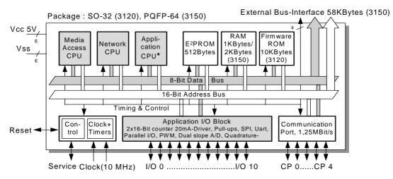
TOSHIBA offer various Neuron IC models in different package types and memory sizes: The model 3120 is a single chip Neuron – no external memory is required; the 3150 is an equivalent to a 3120 with the exception of its external memory interface used to store the firmware, program and application data.
