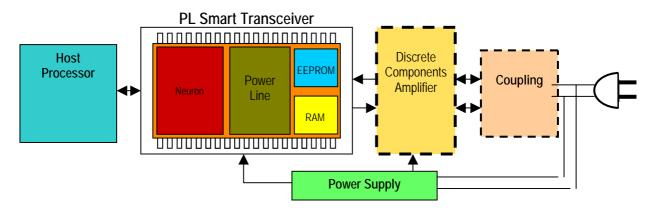
The power amplifier is an around-50 discrete components design (mostly resistors and condensators along with a small number of transistors).
