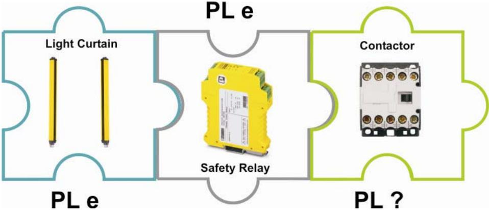
**Figure 1. Safety circuit rated for Performance Level “c”**
