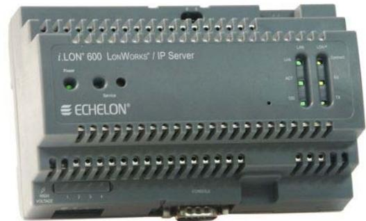
The impressive performances of the iLon-600 come from the successful combination of a powerful RISC 32 bits processor and the Echelon’s *Virtual Network Interface (VNI)* software architecture. Both allow for a high throughput in control networks with large number of nodes, providing high refresh rate of data handling or SCADA displays.
